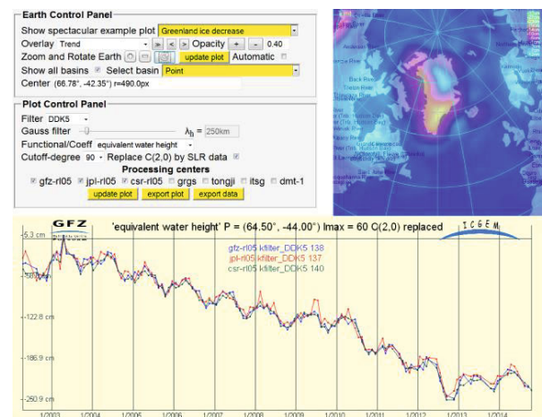
Fig. 3 Snapshot of the G 3 -Browser; the plot shows the time series of the anisotropically filtered (DDK5) monthly solutions from GFZ, JPL and CSR at a point affected by the ice loss in Greenland
